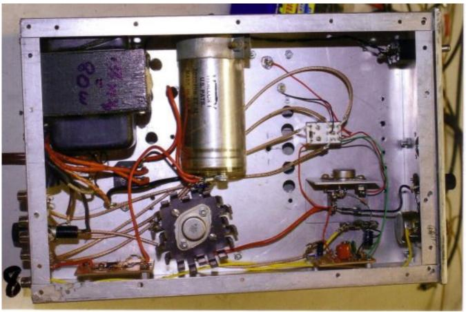
Picture #8: Underneath CCI 20 w Amp. 12v regulated supply, key shaping using PNP transistor, relay to kill amp during transmit
