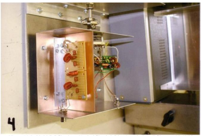
Picture #4: Inside LP/BC filter box. Vertical filter is BC band, stacked small filters are LP 40/20
