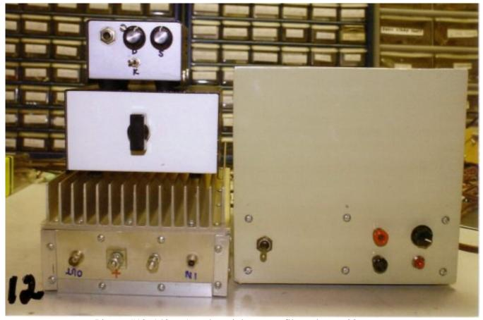
Picture #12: 140 w Amp heatsink, output filters, keyer, 20 w amp
