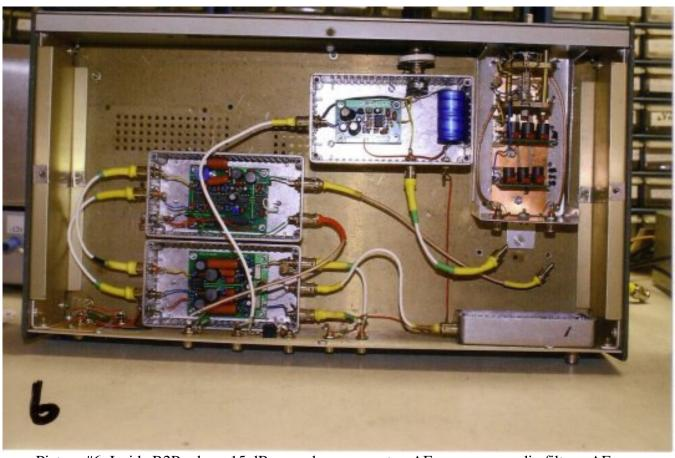
Picture #6: Inside R2Pro box; 15 dB amp, downconverter, AF processor, audio filters, AF amp
