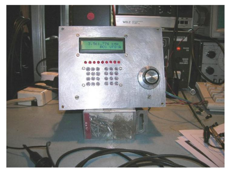
I have not used the IQPro in earnest yet. Originally. the idea was to replace the DDS VFO in a homebrew 9MHz IF 80M Superhet tx/rx (the Plessey SL600 series design of 1973). I guess it would be possible to re-write the PIC code to generate the correct mixing freqs & display the operating freq on the display, but my knowledge of Micro controller programming is restricted to Parallax Basic on the Basic Stamp.
