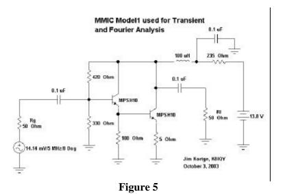
The generator in the simulation model is set to twice the desired input voltage since onehalf of the power is consumed in the generator's internal impedance, Rg. The input of the MMIC model starts at the base of the first transistor and its bias resistors.
